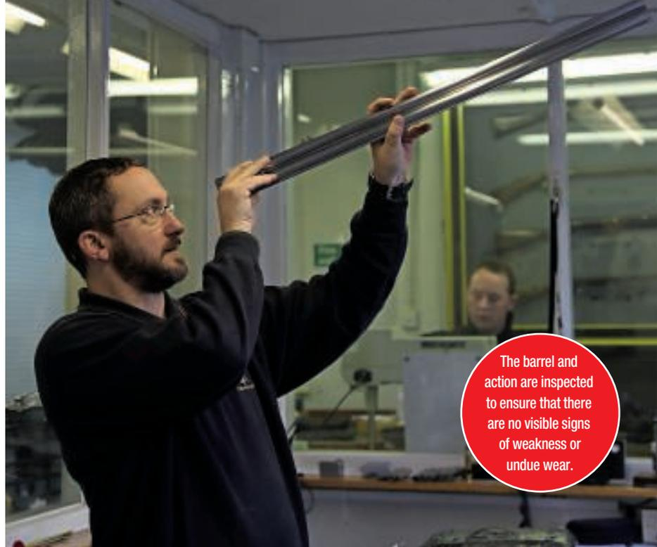
The barrel and action are inspected to ensure that there are no visible signs of weakness or undue wear.
